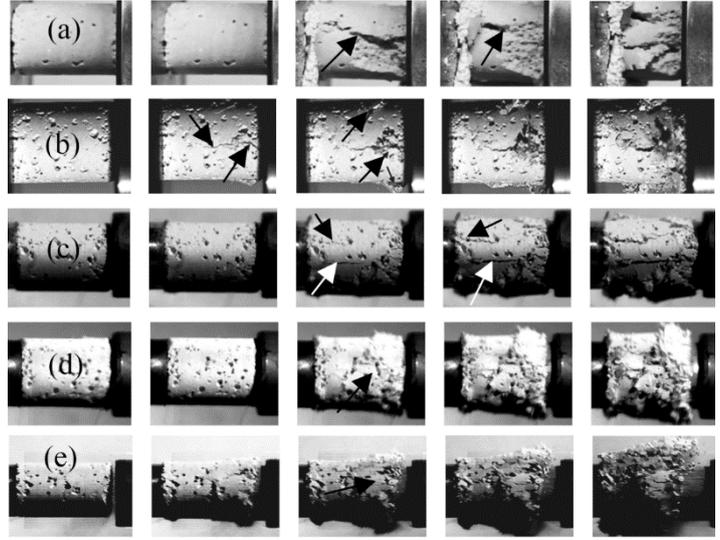
Fig. 3. The deformation pictures of the samples tested at (a)  $5 \times 10^{-5}$ , (b) 1, (c) 10, (d) 30 and (e) 108 m s<sup>-1</sup>
