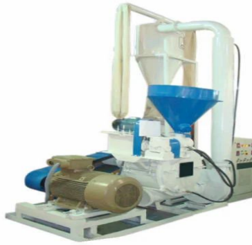
Fig. 4. Laboratory-Scale Mechanical Grinder Used for PVC Size Reduction
