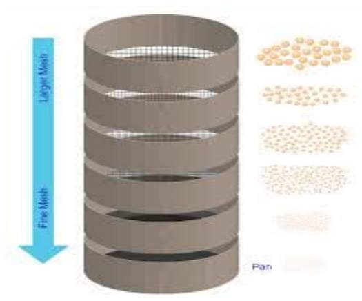
Fig. 5. Stacked Laboratory Sieves Used for Particle Size Analysis of Ground PVC
