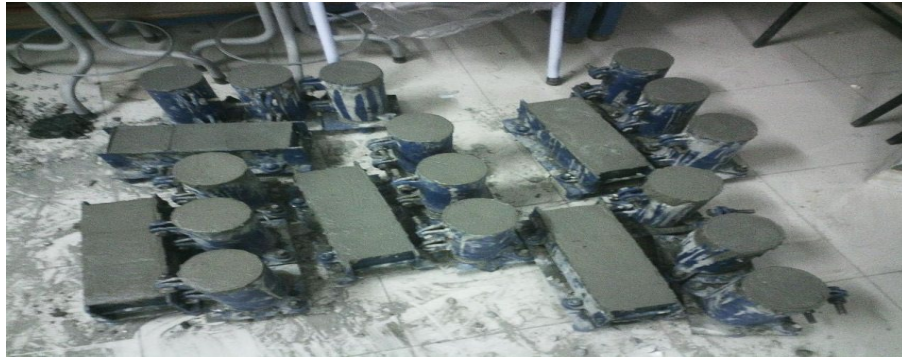
Fig. 8. Cylindrical and Prism Molds Used for SCC Casting
