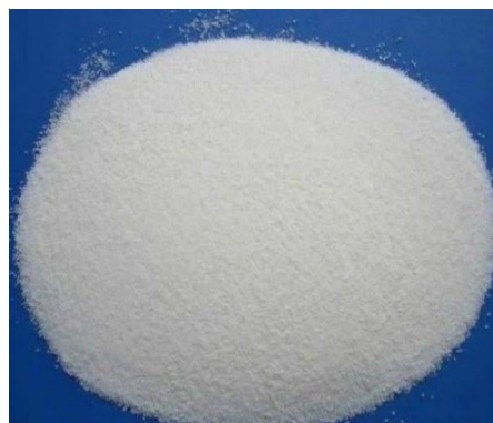
Fig. 6. Pulverized PVC Waste for Self-Compacting Concrete Applications
