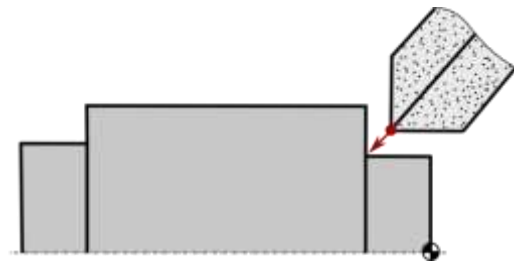
Fig. 12. Plunge grinding of a cylindrical surface and face using CYCLE451
