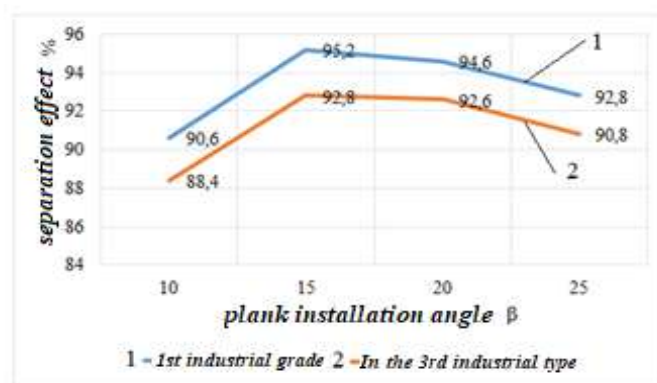
Fig.2. Effect of Slope Angle on Separation Efficiency of Placing Planks Towards the Center of the Separating Drum
