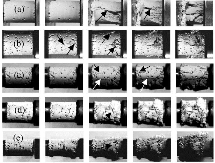
Fig. 3. The deformation pictures of the samples tested at (a) 5 \times 10^{-5} , (b) 1, (c) 10, (d) 30 and (e) 108 m s -1
