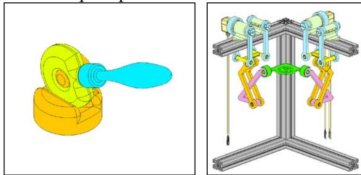
*Fig. 1. a) Three Degrees of Freedom Serial Spherical Manipulator Responsible for Orientations,
