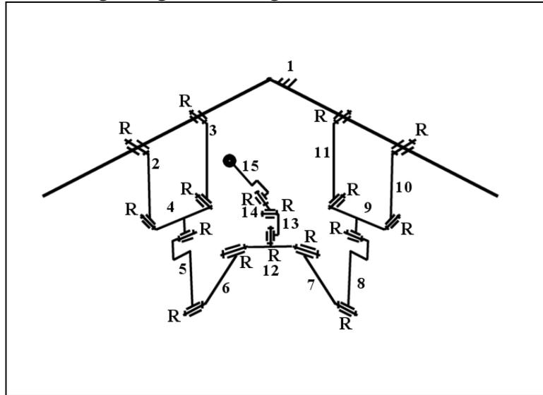
*Fig. 3. Simple Kinematic Structure of Designed Hybrid Manipulator*
