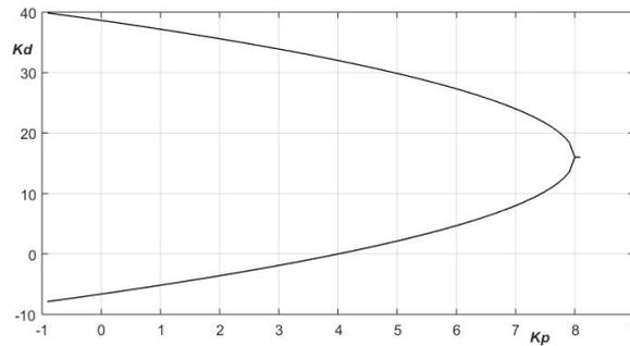
Figure 9. Stability boundary curves for  $k_d = f(k_p)$
