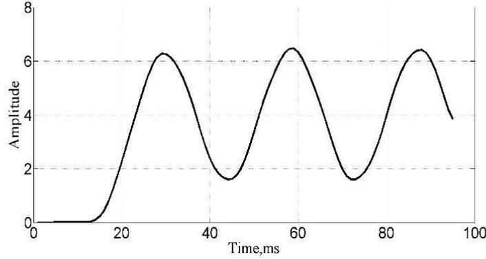
Figure 3 Marginally stable system (Rule 6)
