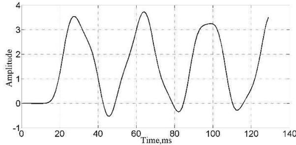
Figure 5 Marginally stable system
